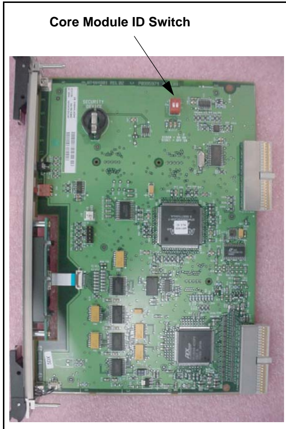
Figure 3 Core Module ID switch
